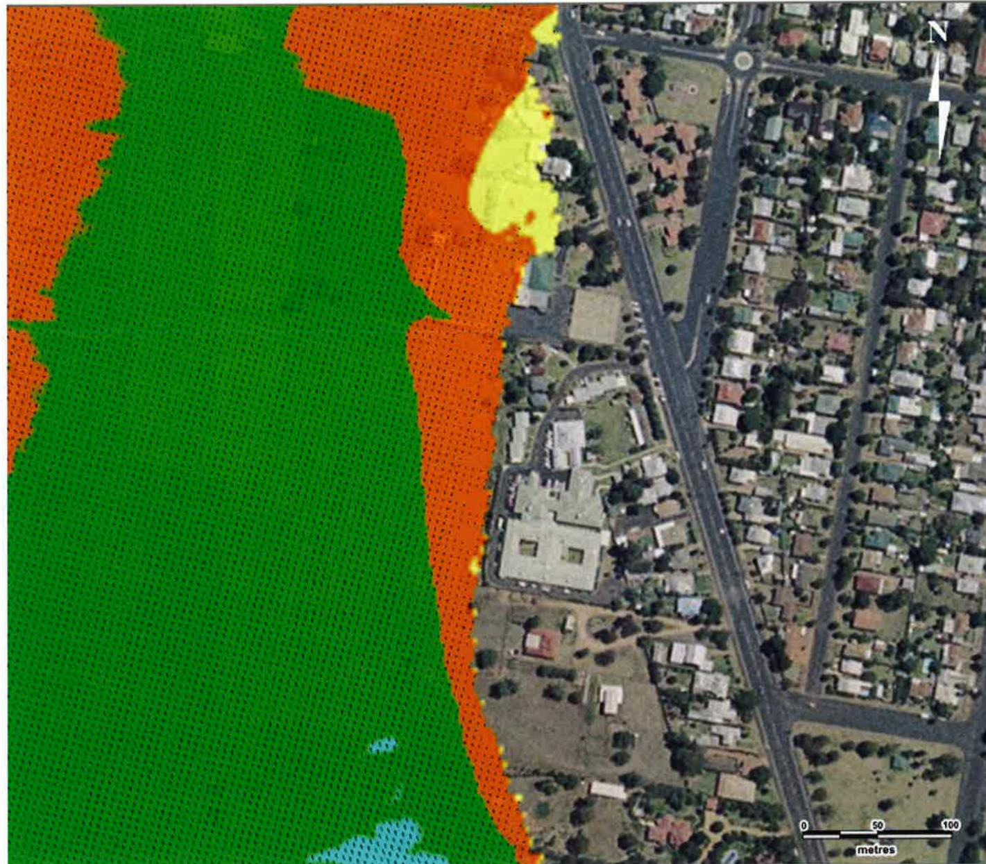
Figure 5 100 yr ARI Flood Velocities – Existing Conditions
