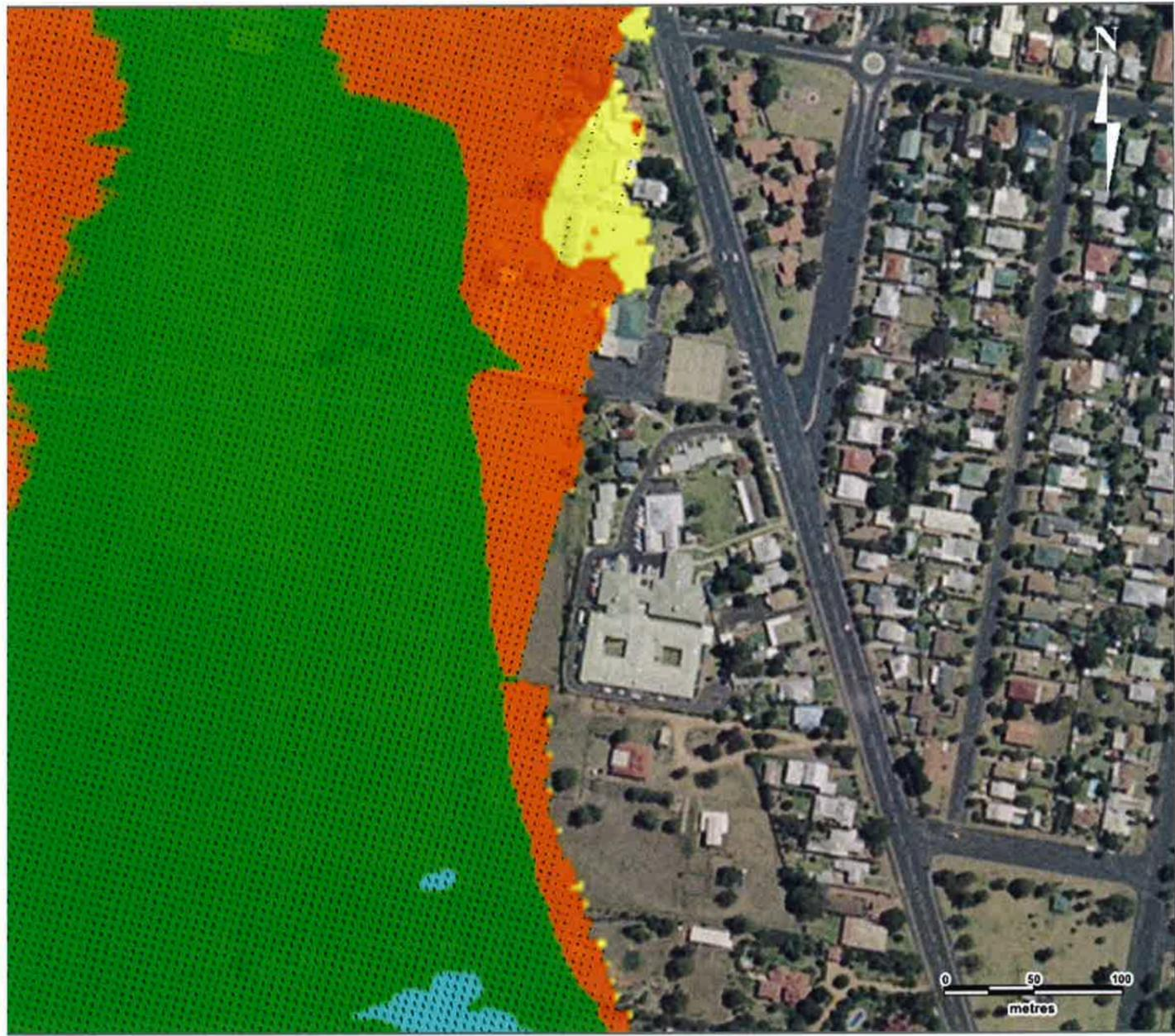
Figure 10 100 yr ARI Flood Velocities - Post Expansion of Bracken House
