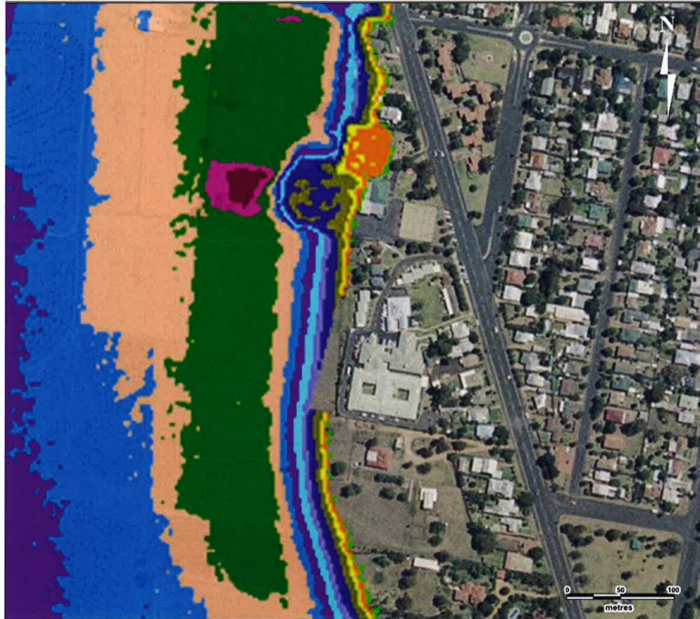
Figure 8 100 yr ARI Flood Depths - Post Expansion of Bracken House
