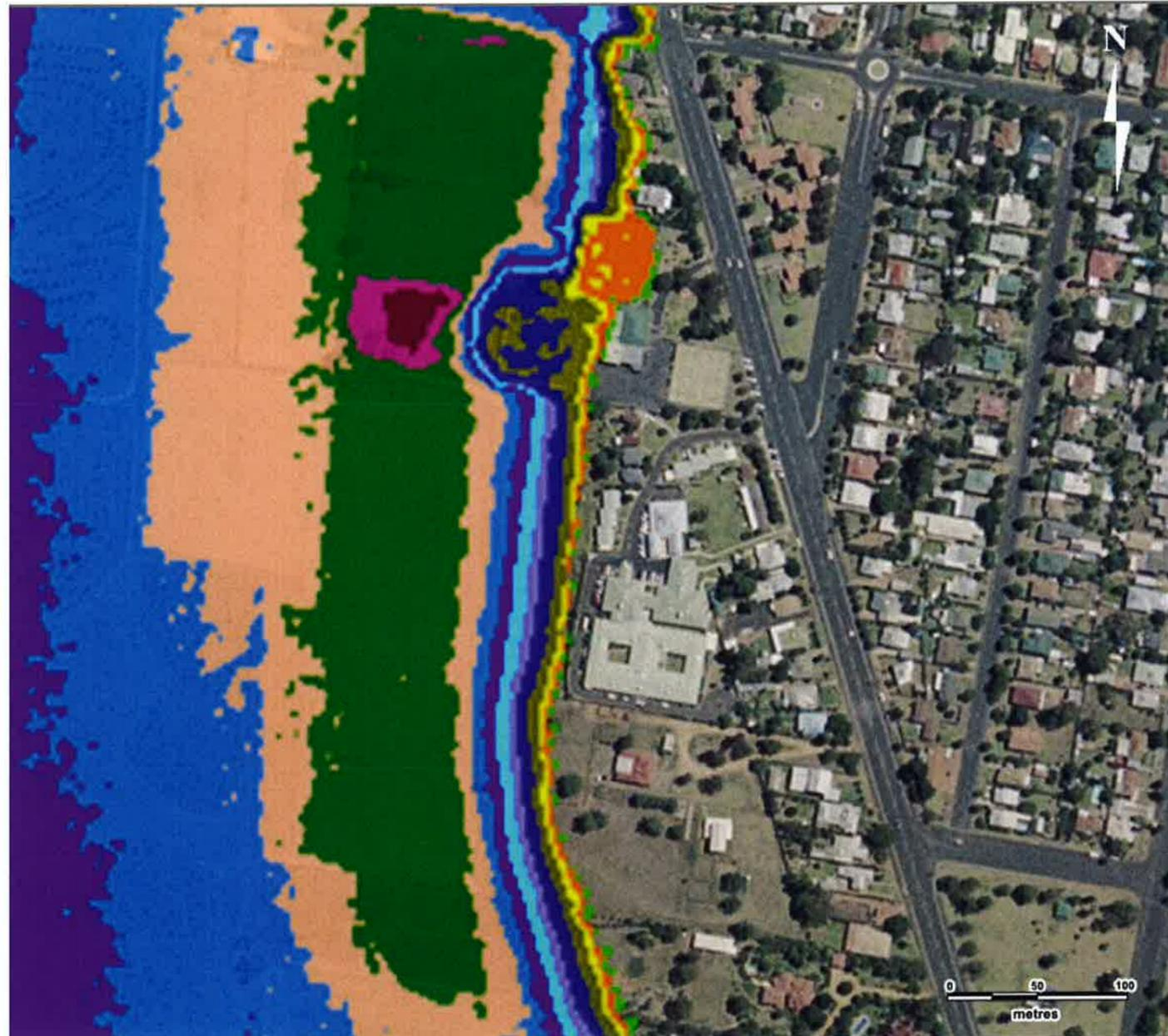
Figure 4 100 yr ARI Flood Depths – Existing Conditions
